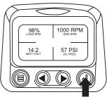
The main menu will pop up on the display. Use the "Arrow Buttons" to scroll through the menu until the "Adjust Backlight" is highlighted.
